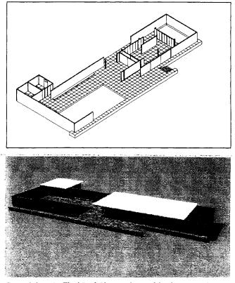
Figure 6: Stage 5 - Third Draft Plan; resolution of details, accommodation to specific architectural objects. Roof omitted. Line Drawing above and fully rendered view below
