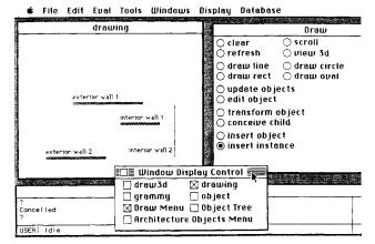
Figure 10: Preliminary representation of walls' geometry: Two exterior walls and two interior walls of Mies' German Pavilion drawing on the left-hand side of the widow below; the instantiation option is invoked in the Draw Menu at right.
